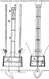
Fig. 7.-Air-lock Diving Bell. A, Working chamber. E. Tackles suspended from roof Air-lock. for raising and lowering
